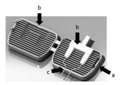
Figure 1. a) Press the wall to unlock. b) Cavity for the connector and back aperture to pass through the adapter cable. c) Front aperture to pass through the electrodes cables.
