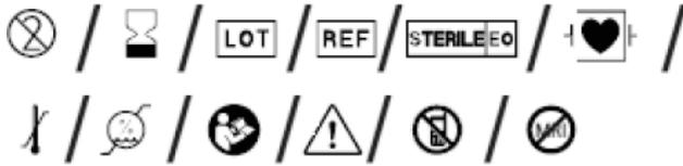
Do not re-use / Use-by date / Batch Code / Catalogue Number / Sterilized using ethylene oxide / CF Defibrillation-proof type of applied part / Temperature limit / Humidity limitation / Follow instructions for use / General warning sign / Mobile phone prohibited / MRI prohibited. You can find the concrete temperature and the humidity limits in the instructions for use, on the box and in the primary pack.
